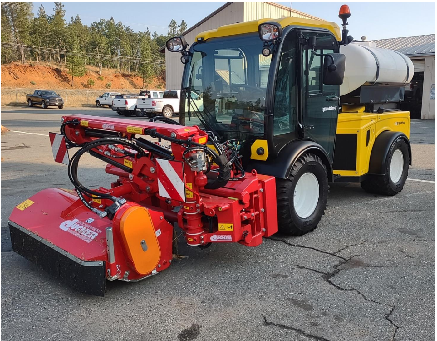
New Multihog with mower attachment and 300-gallon water tank (for fire extinguishing)
